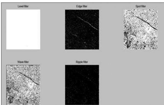
Figure 4: Features extracted using laws mask
